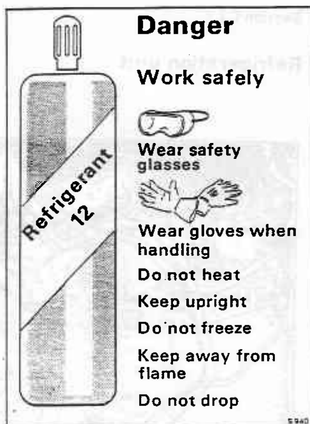
Fig. C3 Refrigerant handling - safety precautions
