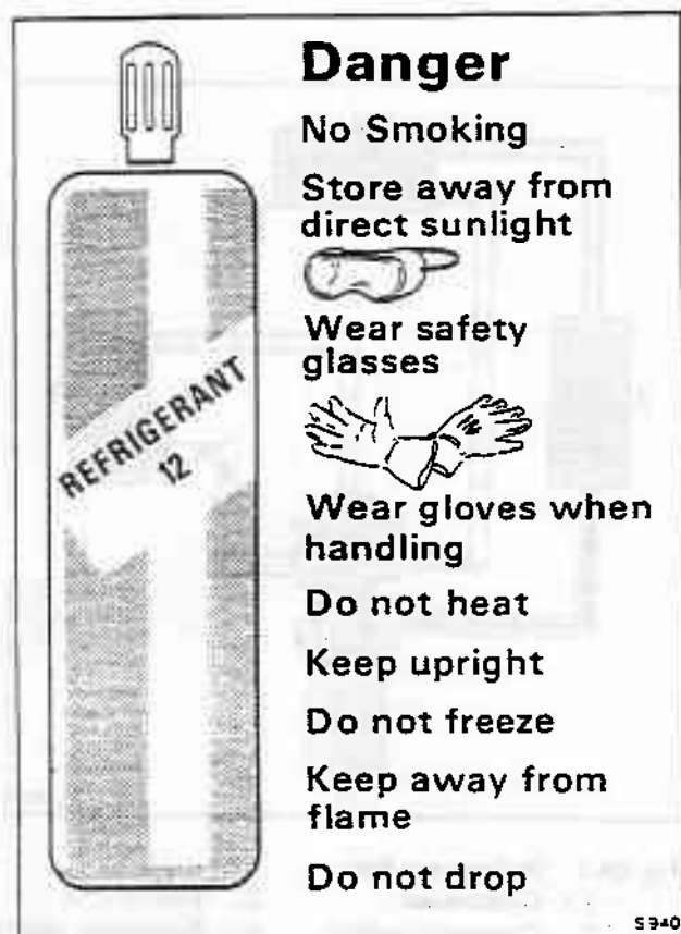
Fig. C6-2 Refrigerant handling – safety precautions
